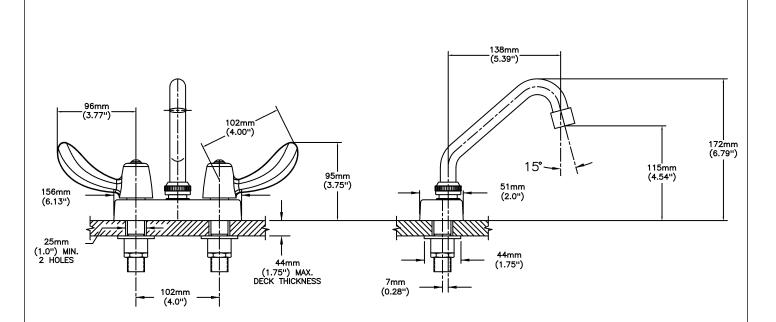
INLET FOR 3/8" OR 1/2" FLEXIBLE RISER OR 1/2-14 NPSM COUPLING NUT (NOT SUPPLIED)
