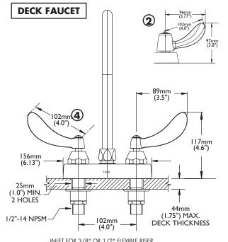
INLET FOR 3/8" OR 1/2" FLEXIBLE RISER OR 1/2-14 NPSM COUPLING NUT (NOT SUPPLIED)
