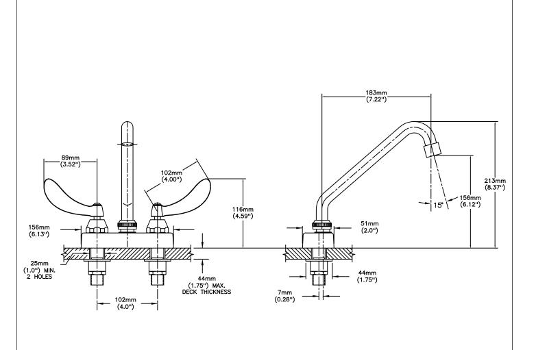
INLET FOR 3/8" OR 1/2" FLEXIBLE RISER OR 1/2-14 NPSM COUPLING NUT (NOT SUPPLIED)
