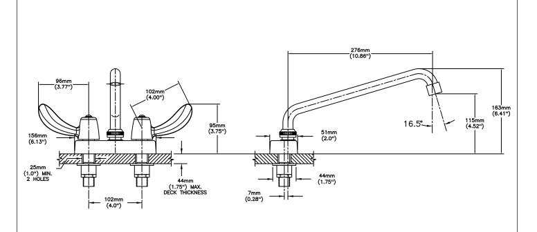
INLET FOR 3/8" OR 1/2" FLEXIBLE RISER OR 1/2-14 NPSM COUPLING NUT (NOT SUPPLIED)
