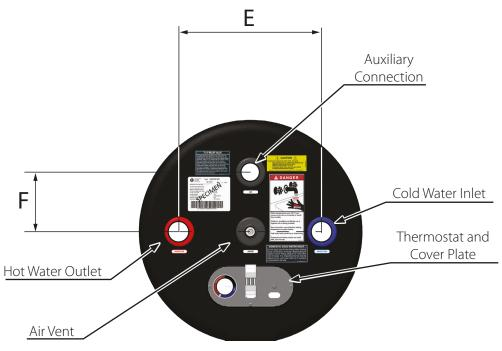
Fig. 27 - SMART Dimensions - Top View
