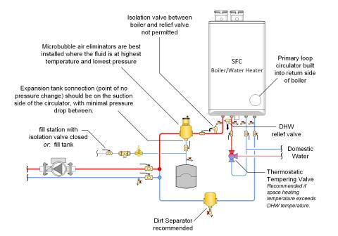
Figure 22: Boiler trim basic options – concept drawing is only a simple schematic guide
