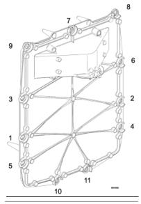
Figure 45: Tighten Allen bolts in cross pattern direction.
