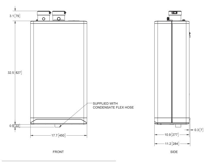
Figure 1a: Dimensions / Connections for SFC Series
