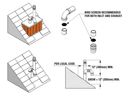
Figure 5b: Rooftop vent terminal configurations
