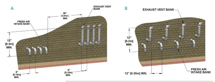
Figure 12: Sidewall vent termination - multiple vent piping configuration
