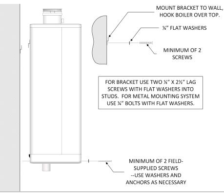
Figure 2: Wall mounting of unit
