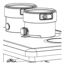
Inlet and outlet vent connections. Note the flue exhaust test port.
