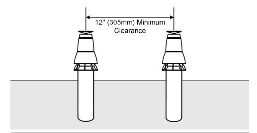
Figure 6: Vertical Concentric Termination - Two Kits
