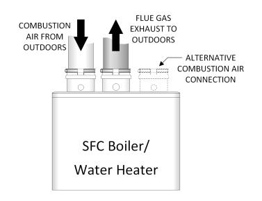
Figure 16: Direct vent combustion air intake
