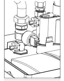
Figure 49: Water Pressure Sensor Type LWCO
