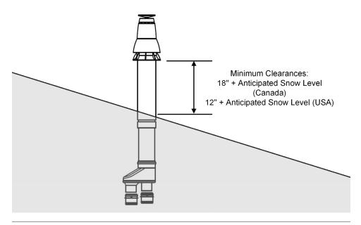
Figure 7: Vertical Concentric Termination - Single Kit
