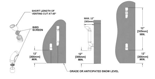
Figure 8: Sidewall vent termination - piping configuration
