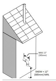
*Figure 5a: Rooftop vent terminal configurations*
