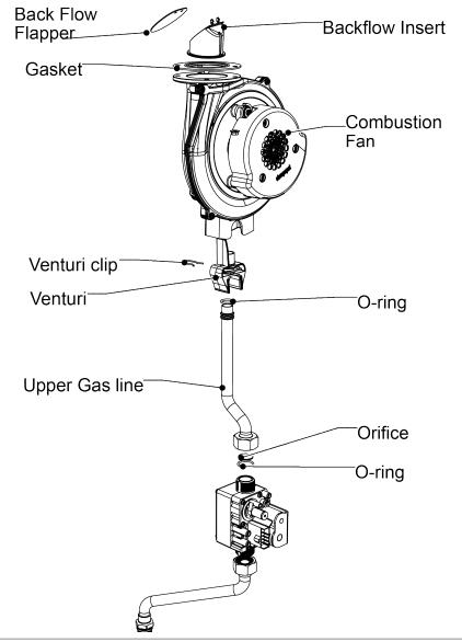
Figure 44: Blower and Gas Valve Assembly
