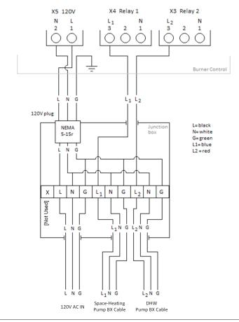
Figure 36: Junction box schematic
