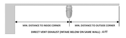
Figure 9: Top view - minimum distance of exhaust vent to inside and outside corners.
