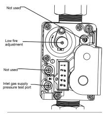
Figure 40 Gas Valve Adjust
