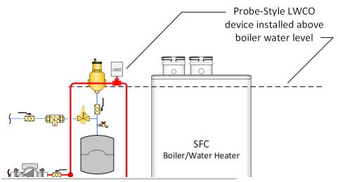
Figure 37: External Probe Type Low Water Cutoff Device
