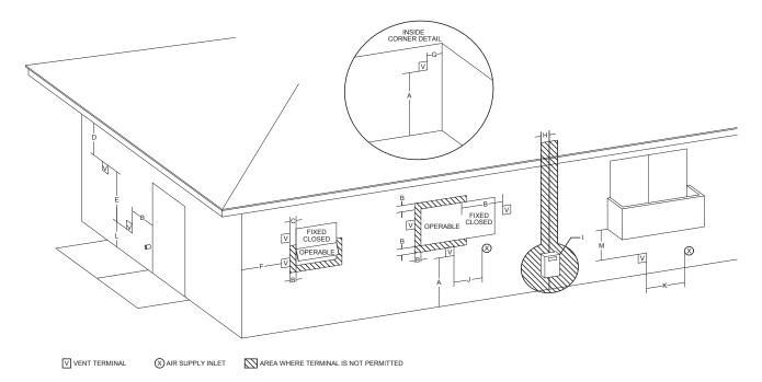
Figure 15: Vent Terminal Clearance
