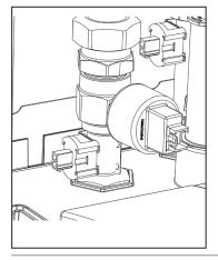
*Figure 48: Water temperature sensor*
