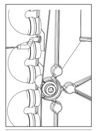
*Figure 47: Heat exchanger temperature sensor*
