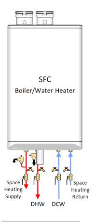
Figure 20: Overview of piping connections
