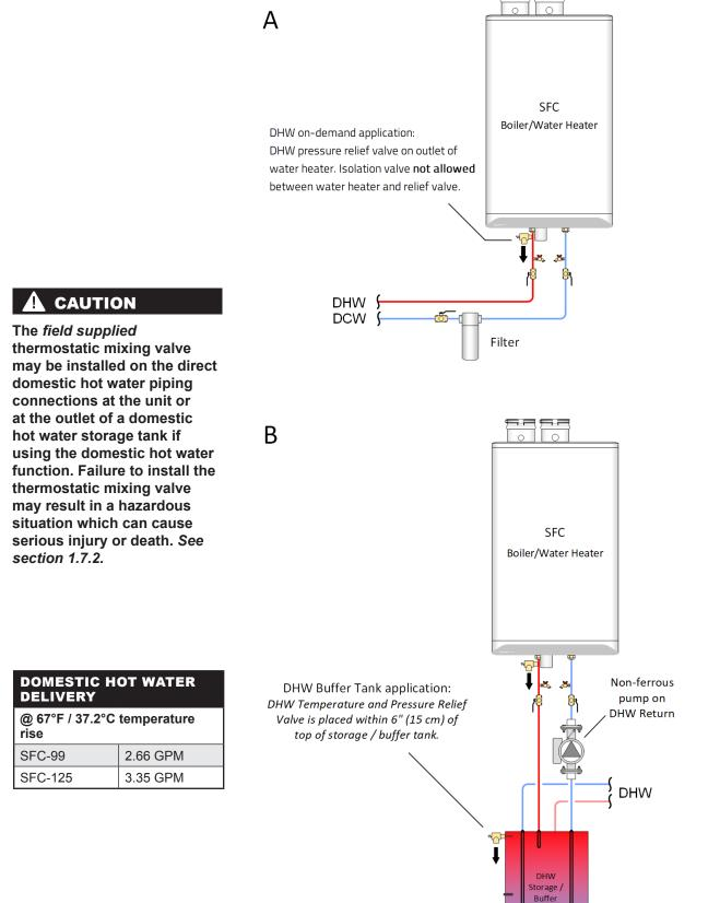
Figure 31: Tankless DHW Piping Options – concept drawing. This drawing is only a simple schematic guide.
