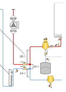
*Figure 24: Basic Primary/Secondary piping with closely-spaced tees concept – concept drawing. This drawing is only a simple schematic guide.*
