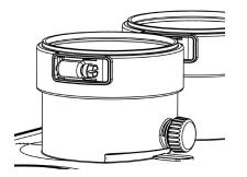
Figure 41: Flue gas test port plug
