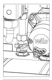
Figure 50: Domestic Water Flow Sensor
