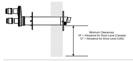
Figure 11b: Horizontal Concentric Termination - Single Kit
