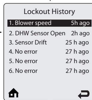
Lockout Details displays the lockout at the top of the screen followed by a snapshot of the boiler information recorded at the time of the lockout.
