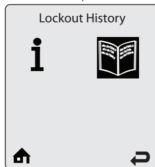
Lockout History displays the last eight lockouts. The newest lockout is displayed at the top of the screen.
