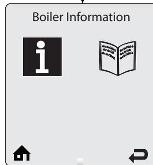
Boiler Information displays six boiler readings at a time. Each line contains an information item followed by its current value. Touch the and soft key to scroll through additional information items.
