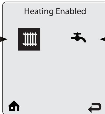
Heating Operation can be enabled and disabled by selecting the radiator icon and touching the
