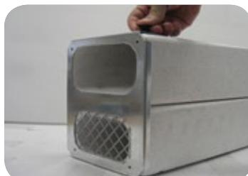
Attach both transition ducts together by inserting them to the transition plate connector. Fasten all 4 vinyl panel retainers into place to secure duct transitions to transition connector plate.
