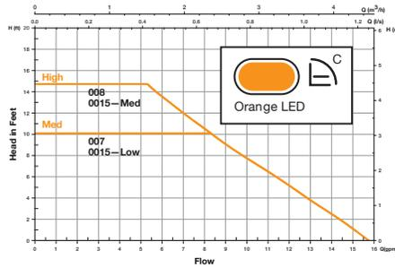
In constant pressure mode (ZV), the circulator maintains a constant pressure differential ( $\Delta p-c$ ) in the system as heating load increases or decreases. Selections options are Medium or High.
