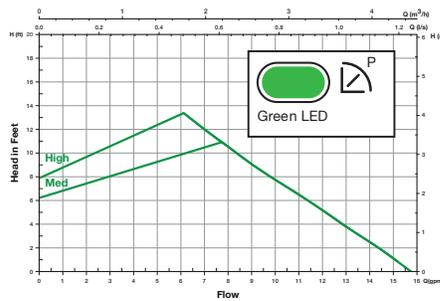
In proportional pressure mode (TRV), the circulator maintains a proportional pressure differential ( $\Delta p-v$ ) in the system as heating load increases or decreases. Flow will change in relationship to the change in pressure differential. Selections options are Medium or High.
