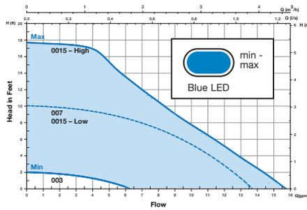
Fixed speed mode (Zone Circ) allows the installer to fine tune the circulator flow rate to precisely match design load conditions. It is infinitely variable between MIN/MAX settings.
