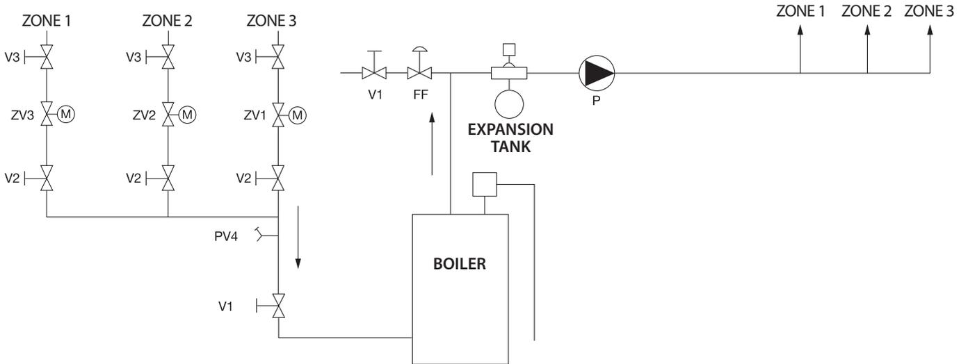
**PREFERRED PRIMARY / SECONDARY PIPING FOR ZONE VALVES ON BOILER SUPPLY**
