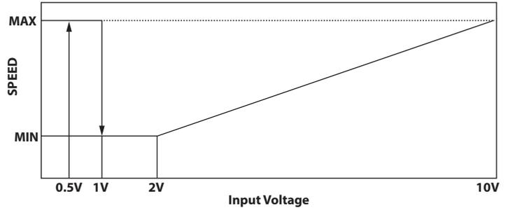
**IMPORTANT: If the input remains disconnected, the circulator runs at max. speed**
