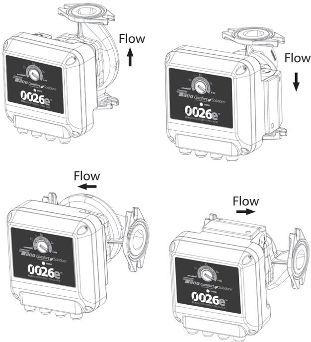
**Figure 5 — Unacceptable Mounting Positions**
