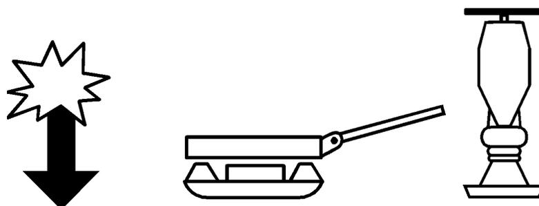
Static Compactors (Figure 5-4): Consolidation with static compactors occurs as a result of the rolling weight of the equipment itself. Sheeps-foot rollers employ projecting feet to concentrate the weight of the machine. Static compactors are most valuable when used on non-cohesive backfill away from the pipe. Other methods of compaction should be used near the pipe.
