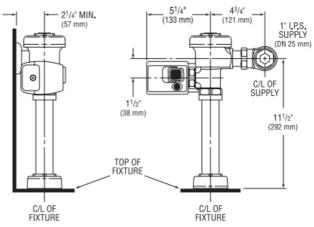
Side Mount Operator unit shown on an existing Sloan Regal Model 110/111 Closet Flushometer
