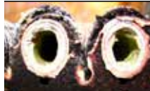
Scale buildup from untreated water.
