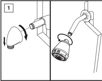
**1. Connect to elbow (RP36004 not supplied), or remove existing shower head.** Turn the existing shower head counter-clockwise with adjustable wrench or pliers. Use care not to unscrew the shower arm; hold the shower arm secure. **NOTE:** If your shower arm has a ball on the end of it, it will not work with this shower unit and will need to be replaced with a standard shower arm.
