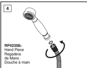
**4. Connect tapered end of hose to hand shower.** Seat the washer, if provided, firmly into the hose nut. Carefully align the thread of the tapered end of the hose directly to the hand shower. **Hand Tighten—do not use a wrench or pliers.** Then place the hand shower into the wall mount holder.
