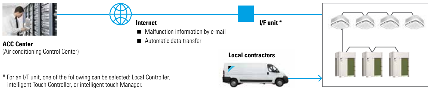
D-NET Air Conditioning Network Service System overview
