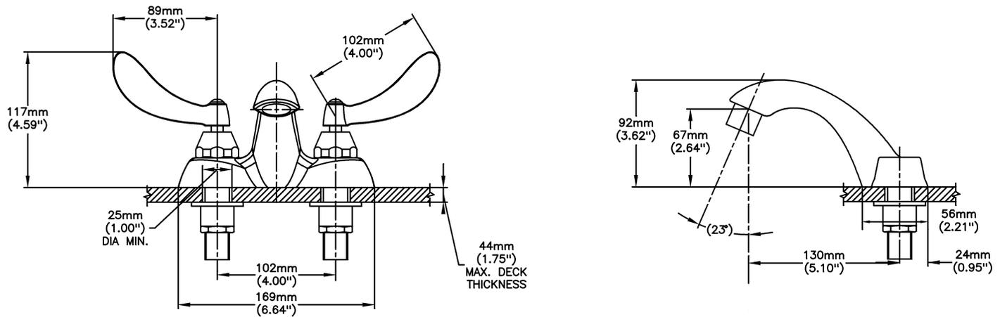
INLETS: 1/2" MIP/COUPLING NUTS (NUTS NOT SUPPLIED)
