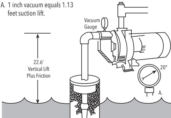
A reading of 20" on a vacuum gauge placed on the suction side of the pump would tell you that you had a vacuum or suction lift of 22.6 feet.
