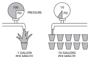
Now as to the resistance to flow which will be encountered, there are three causes. These are (1) the resistance by the outlet itself such as a partially rusted shower head, (2) friction loss in pipe lines, and (3) that resistance due to difference in elevations.
