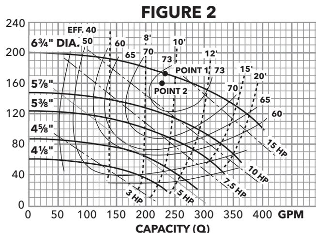
Determine that the new impeller will meet the required capacity:
