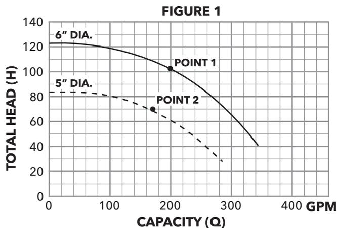
The 5 inch diameter Head/Capacity performance point can be plotted on the graph (figure 1; point 2). By taking additional Head/Capacity points on the 6" diameter curve and using this procedure, a new Head/Capacity curve line can be produced for the 5 inch diameter impeller.
