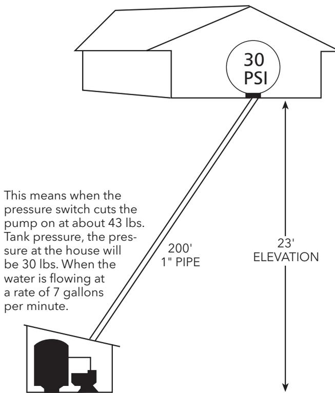
This means when the pressure switch cuts the pump on at about 43 lbs. Tank pressure, the pressure at the house will be 30 lbs. When the water is flowing at a rate of 7 gallons per minute.
