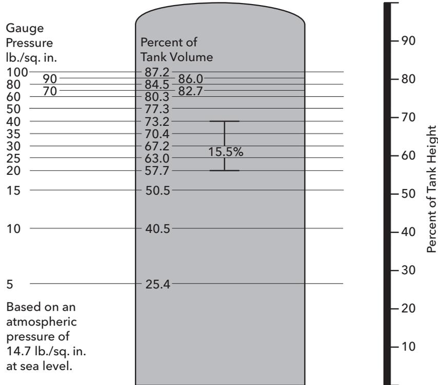
When using large standard galvanized tanks, a constant air cushion is required for proper operation of the water system.
