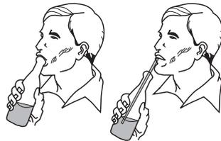
Try to lift soda from a bottle by closing your mouth over the mouth of the bottle. It can't be done. When you use a straw, it is easy - you are creating a partial vacuum in your mouth, exposing the surface liquid to atmospheric pressure, the difference in pressure raises the liquid.
