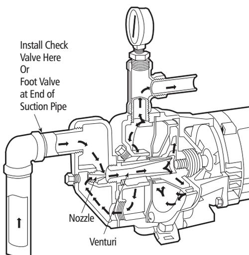
In shallow well jet pumps the jet assembly is built into the pump casing as in the Goulds Water Technology J5S. Or, the jet assembly, shallow well adapters, can be bolted to the centrifugal pump. In either case there is only one pipe extending into the well . . . the suction pipe.
