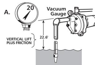
A reading of 20" on a vacuum gauge placed on a suction side of the pump would tell you that you had a vacuum or suction lift of 22.6 ft.
