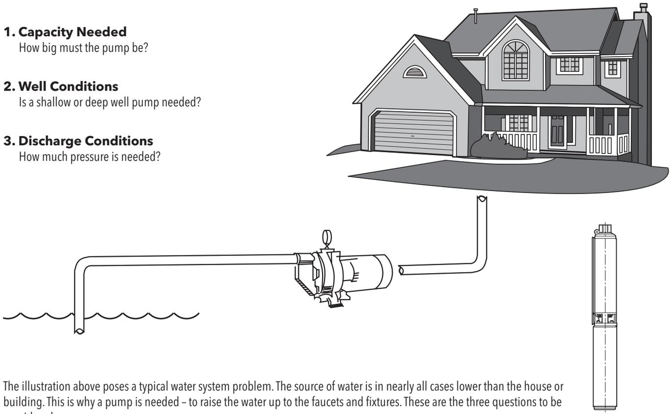
The illustration above poses a typical water system problem. The source of water is in nearly all cases lower than the house or building. This is why a pump is needed – to raise the water up to the faucets and fixtures. These are the three questions to be considered:
